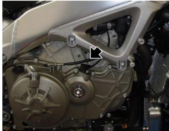
**GE / REMPLACER LE CAPTEUR, S'IL EST OK, TESTER LES BROCHES 20 ET 35 DU CONNEXEUR ENGINE DU BOÎTIER MARELLI.**
