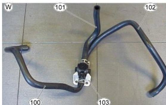
**TABLEAU X - MONTAGE ET BRANCHEMENT DU CONNECTEUR DU SOLÉNOÏDE D'AIR SECONDAIRE ET MONTAGE DU COLLECTEUR EN CAOUTCHOUC AVEC COLLIER CLIC**
